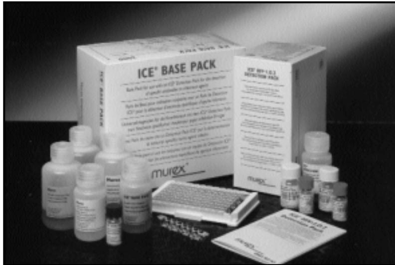
A UK-produced ELISA test kit from Murex including rack of testing wells (centre)
